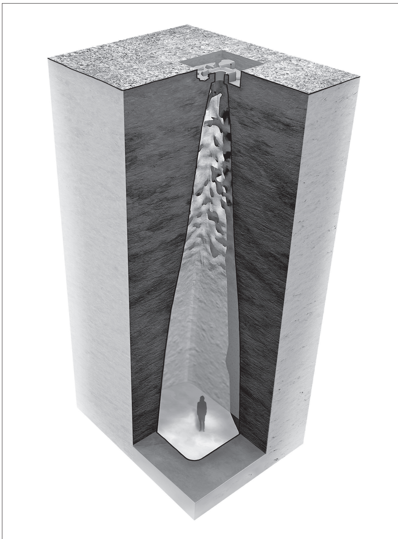
7. 3D architectural model of the Hasmonean cistern: length 4.72 m; width 9.32 m; min. height 14.9 m; max. height 15.7 m; full capacity 110,000 litres \approx 29,000 US gallons
